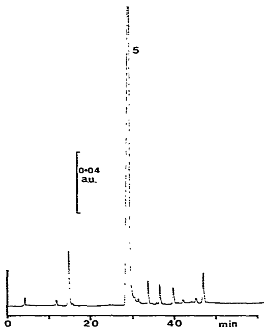
Fig. 4. HPLC elution profile of desulphoglucosinolates isolated from mustard seed ( Sinapis alba ). The peak number refers to the glucosinolate listed in Table I. Chromatographic conditions are described in the text.
